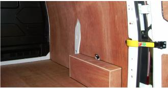
Kits consists of 6 mm plywood on the sides & door panels and 12 mm plywood on the floor & wheel arches. Van openings are finished with aluminium door trim & all edgings are finished with silicone sealant.
